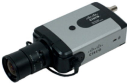
Figure 1. Cisco 2600 IP Camera Shown with Optional DC Auto Iris Lens
